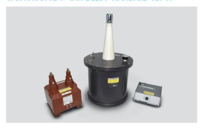
This setup includes an SF6 gas-filled Standard Capacitor, a Step-down Voltage Transformer (11kV/110V), and a Dissipation Factor Error Standard. It can introduce Tan Delta values from 0% to 10%, making it suitable for calibrating Capacitance and Tan Delta Test Sets up to 10kV. Additionally, Eltel offers a portable 15kV C&DF calibrator for both in-house and on-site calibrations, with a CMC of 0.61 pF for Capacitance and 0.014% for Tan Delta
