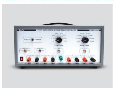
The CVRPS 2013 standard generates fixed Ratio and Phase Errors across the entire range, enabling the calibration of Instrument Current Transformer Test Sets and Voltage Transformer Test Sets using the Direct Method. This unique standard, available only at Eltel Industries, ensures a Class-leading CMC of 80 PPM and 0.3 minutes. It is currently unavailable in other NABL accredited labs
