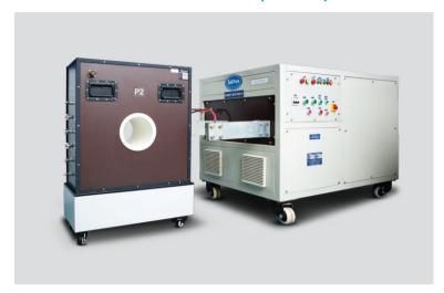
Eltel's Precision Current Transformer, paired with a 7200A High Current Source, covers ratios from 5A/5A & 1A up to 6000A/5A & 1A, with an overall uncertainty of 96 PPM — comparable to the best calibration labs worldwide. This range supports the calibration of both standard and commercial-grade Current Transformers
