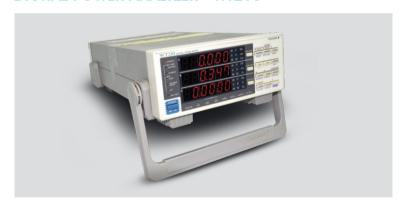
The WT210 Power Analyzer, with a best uncertainty of 0.25%, is used to calibrate Current and Voltage Transformer burdens at 50Hz and 60Hz
